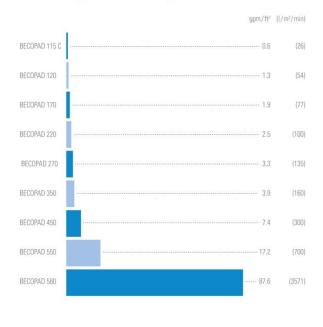
Conditions:  $\Delta$  p = 14.5 psi (100 kPa, 1 bar), Medium: Water at 68 °F (20 °C)
